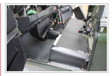
Now install the seat box surround. You will probably need to remove the leather strap and the under-seat storage plate fixings and replace them back once the hardura has been bonded into place. This will achieve the best result, rather than cutting the panels.
